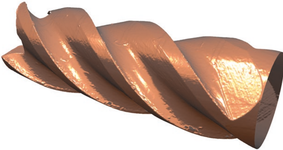
Figure 1 shows the total 3D measurement of an endmill taken with the S neox Five Axis. This measurement provides a complete view of the endmill's surface, allowing for accurate analysis and assessment.
