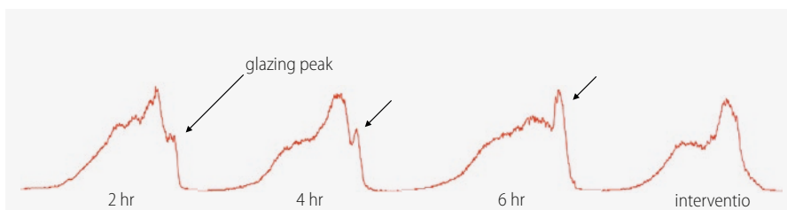
Figure 8. Image showing evolution of the pad asperity height during the polishing process. After several hours of polishing a 'glazing peak' appears in the surface distribution. By monitoring the pad surface at intervals during the polishing process, the pad surface can be duly conditioned (intervention) in order to revert the surface condition to the initial state.
