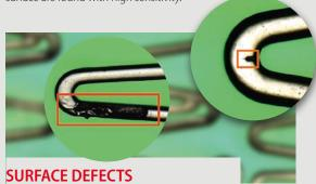
Surface irregularities related with material inclusions, contamination, or polishing defects are seen as contrast changes in either surface of the device. Surface defects detection methods are adapted to brightfield and grazing illumination configurations.
