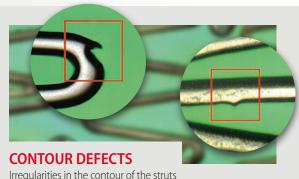
Irregularities in the contour of the struts arising from the laser cutting process or from material inclusions in the lateral surface are found with high sensitivity.
