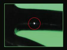
Q vix illumination system is based on high efficiency LEDs and is fully integrated into the sensor. Its flexible design makes possible numerous configurations using up to 7 independent light sources. Standard brightfield illumination setups can be combined with grazing illumination setups, which allows Q vix to detect tiny defects that can be seen "shining in the dark", even at low magnifications.
