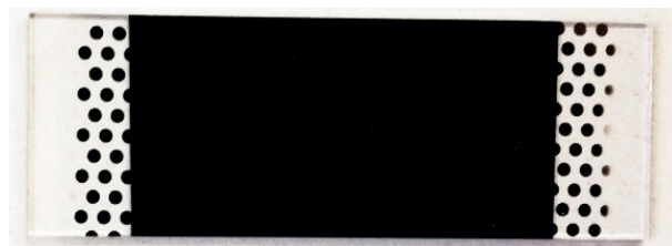
Figure 2. Sample used to determine the thickness of the coating.
