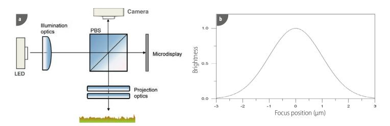
(a) Optical diagram of S mart sensor; (b) Pixel axial responser
