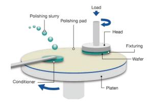
CMP process schematic diagram
