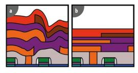
Wafer manufacturing without CMP (a) and with CMP (b)
