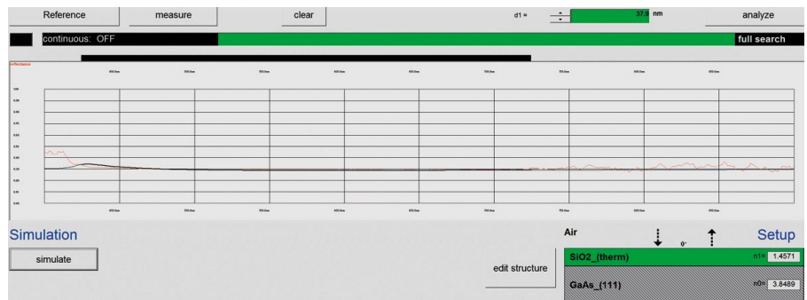
Figure 3. Reflectivity spectrum of a thin SiO 2 film, with model fit showing the thickness (38±1 nm).
