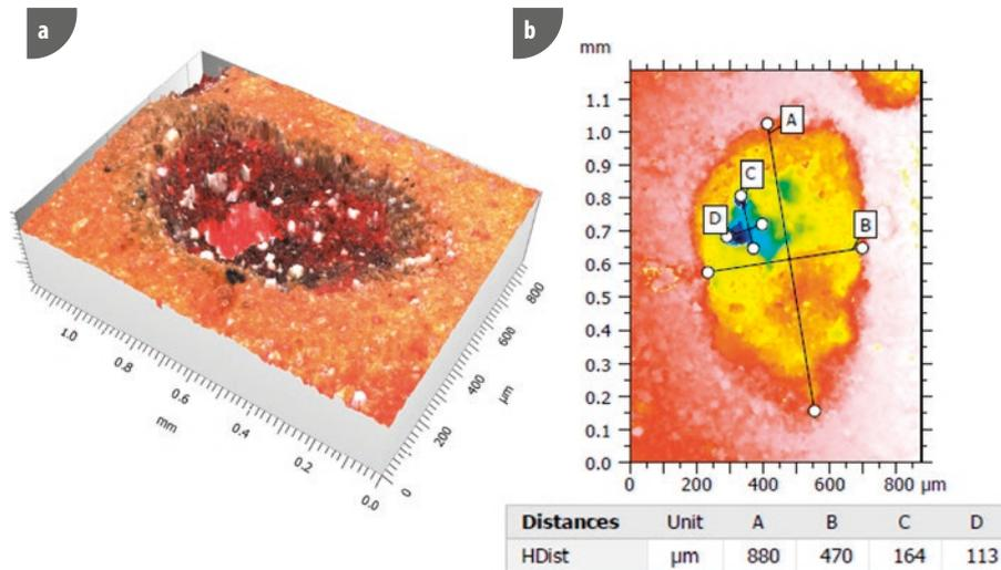
**Figure 4.** Crater formed by 20 shots. a) 3D view of the crater formed by 20 shots;
