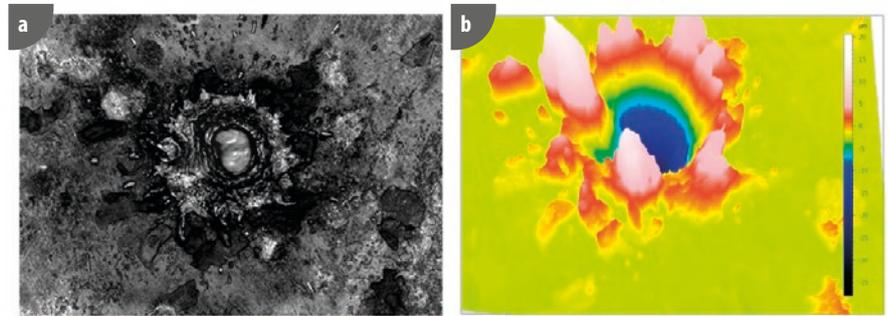
**Figure 7:** Crater obtained after 20 shots with the laboratory instrument, the matter ejections are visible **a)** Image taken with the confocal microscope S neox; **b)** 3D view of the crater.
