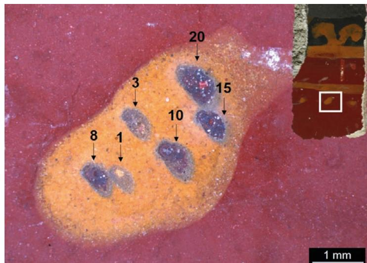
**Figure 3.** Location of the points analyzed at the level of the yellow decor overlaying the red pigment.
