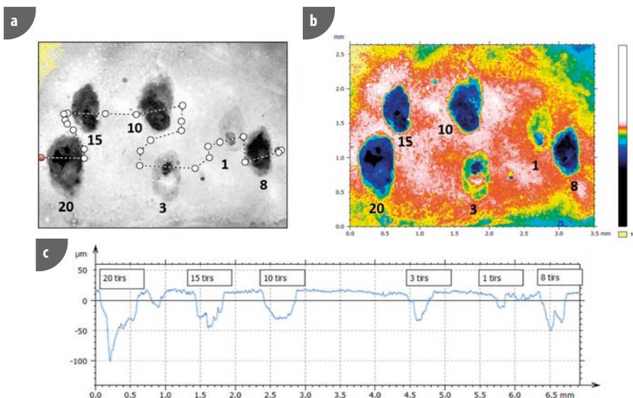
**Figure 5.** Depth of the craters in  $\mu\text{m}$ . a) and b) top-view topographies, c) profile.
