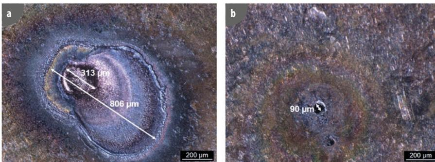
**Figure 9.** Shape and size of the craters; a) Crater obtained after 500 shots with the portable instrument (EasyLIBS); b) Crater obtained after 500 shots with the laboratory instrument.
