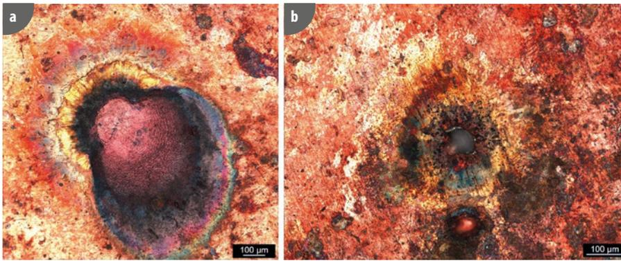
**Figure 8.** a) Crater obtained after 50 shots with the portable instrument (EasyLIBS);
